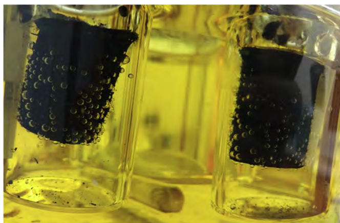
Fig. 9. The bubbling effect; GAL sample showed a large number of bubbles on the surface generated by gasses released during reduction.
